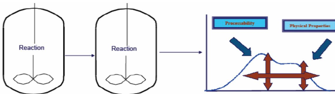
**Figure 2 Dual Reactor Bi-Modal PE4710 Technology<sup>1</sup>**
